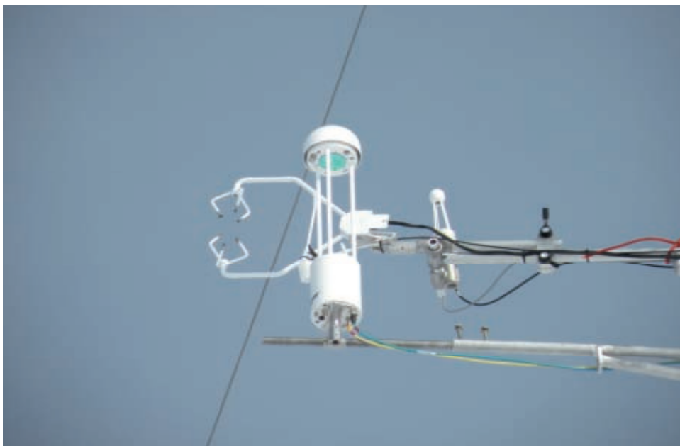
Set up of the eddy covariance system and the open path gas analyzer at 20 m on the CCT
