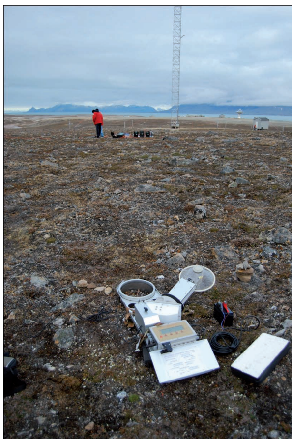
Figure 4 CO 2 fluxes measurements in one of the 6 plots selected within the CALM grid and close to CCT tower. On the background the ERT instrumentation, the CCT tower and the Ny-Ålesund airstrip
