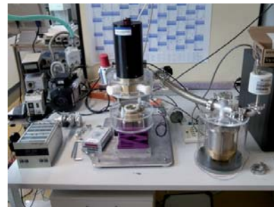
Figure 2: IN counter FRIDGE.
