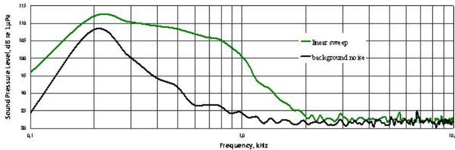
Figure 1: Mean power spectrum of sweep signal and background noise. The sampling frequency of the signal was 100 kHz. The size of Fast Fourier Transform (FFT) was 1024 points and the window type was cosine tapered.
