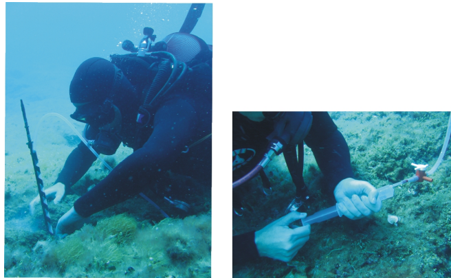
Figure 5: Water and dissolved gas sampling from submarine fluid discharge.
