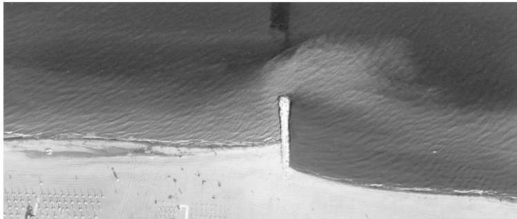
Figure 5: Example of suspended sediment (turbidity) around a groin located in the Adriatic sea.
