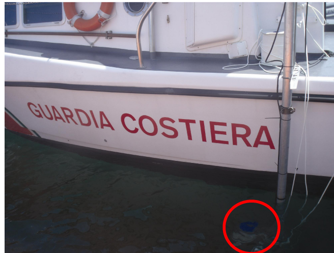
Figure 4: The ADCP mounted on the left side of the Coast Guard patrol boat is visible in the water in the red circle.
