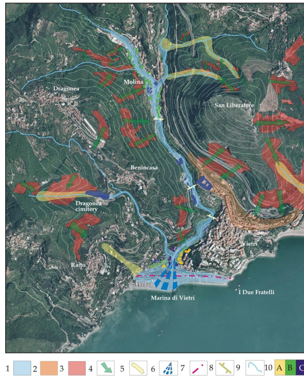
Figure 5: Geological effects and damage pattern induced by the 1954 flood event. (1) Overflowing area, (2) mud deposits, (3) evidence of past denudation, (4) landslide phenomena, (5) channelled debris flow, (6) alluvial fan, (7) shoreline before 1954 event, (8) temporary dam, (9) drainage network, (10) damage categories: (A) heavy, (B) medium, (C) light [15].
