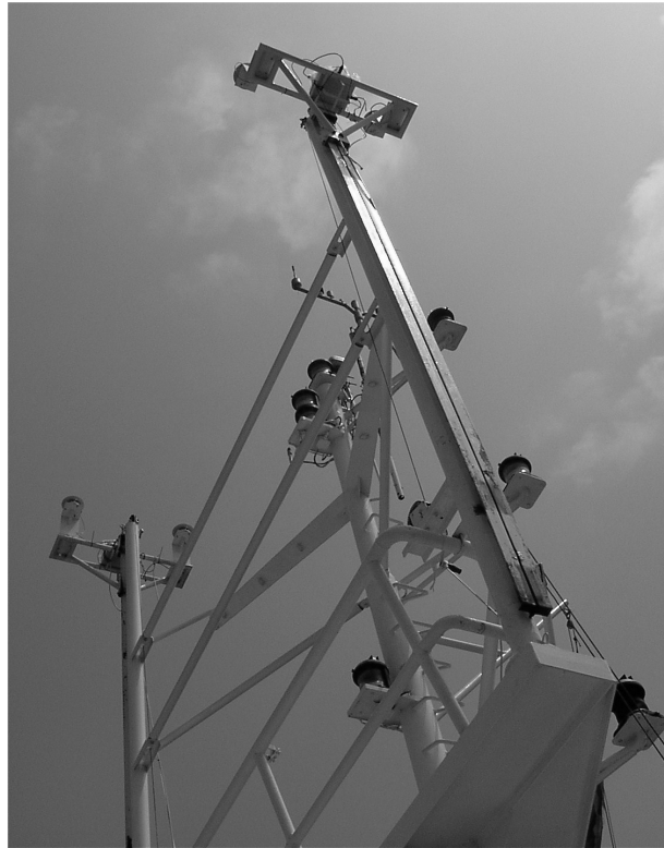
Figure 1: Sensors for meteorological and radiative measurements installed on board the R/V Urania.
