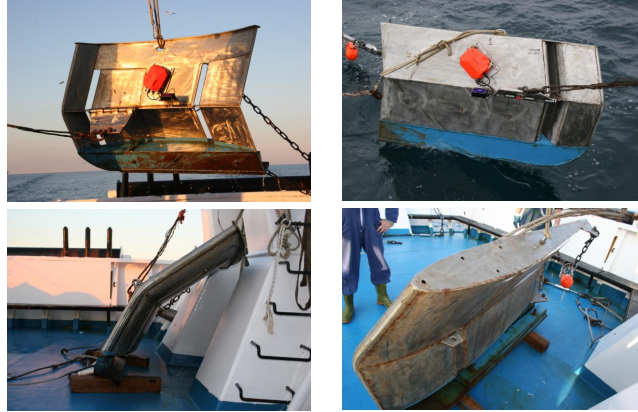
Figure 2: Particular of the Cambered vee AR (on the left) and Clark-Y (on the right) otterboards. Pictures on the top show the SCANMAR angle sensor mounted on the otterboard for measuring heel- and pitch-angles of the door.
