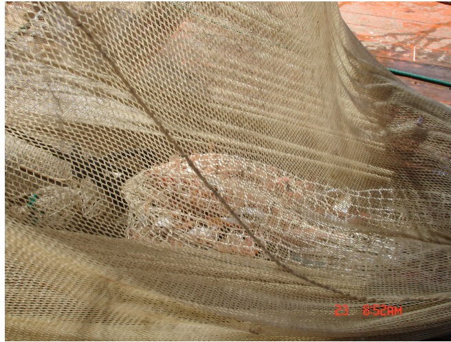
Figure 2: Cod-end and cover on board.
