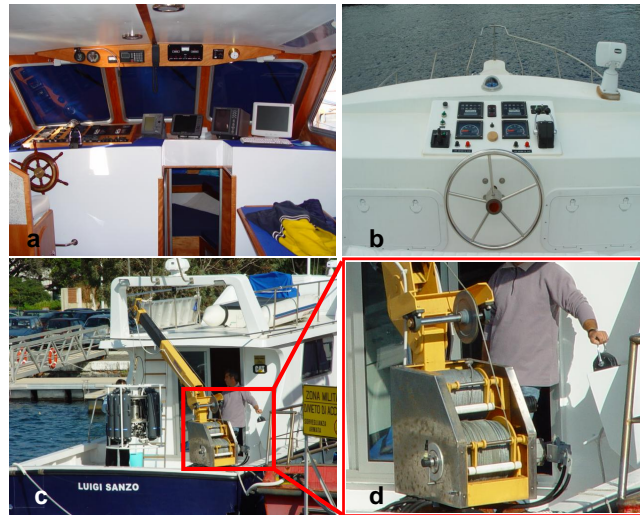
Figure 2: The steering commands: in the cockpit (a), on the upper deck (b), astern near the crane (c), and particular crane/winches (d).
