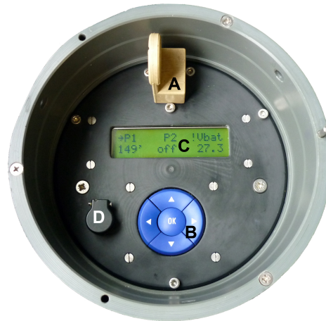
Figure 2: Front panel of the electronics control within the waterproof case (C in Figure 1), which also contains the battery pack. A) magnetic key for programming the control system, B) keyboard for entering commands, C) display, D) connector for charging batteries.
