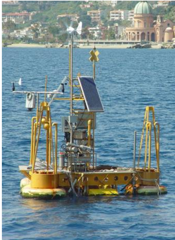
Figure 3: A buoy near Messina. The wind generator is evident on the top, under it the radar reflector, the solar panels, the pumping system on the deck, on the left, the meteorological station
