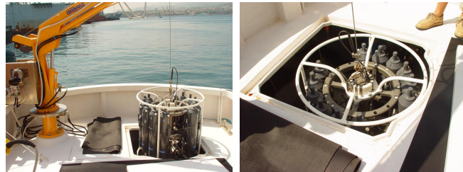
Figure 4: Afterpeak locker of stern with the rosette housing.
