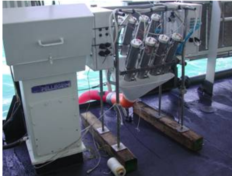
Figure 5: The launcher on the deck of Magnaghi Ship; the eight launch tubes are evident on the right, together with the boxes containing the electronics and the electropneumatic valves
