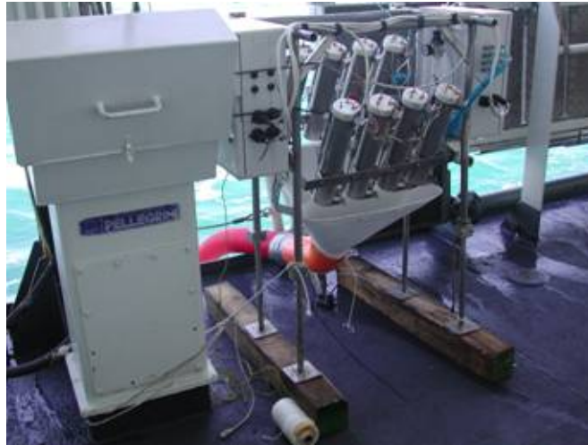
Figure 9: The multiple launcher installed on the deck of the Magnaghi ship.
