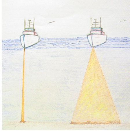
Figure 1: Difference in bottom coverage between singlebeam and multibeam systems.
