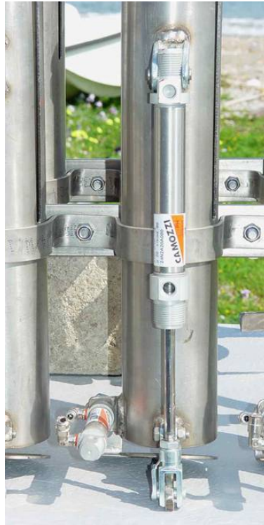
Figure 1: A close-up view of a launch cylinder with the pneumatic actuators during the assembly. The small pneumatic cylinder at the bottom locks the launch door, the vertical bigger one operates it.
