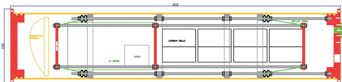
Figure 3 Sketch of the light-weight payload used to study stratospheric circulation in the Arctic during the polar winter (dimensions in mm)
