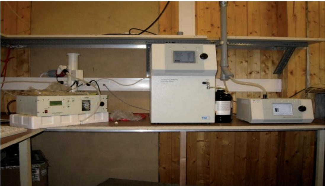
*View of the aerosol samplers set up in the Gruvebadet laboratory*
