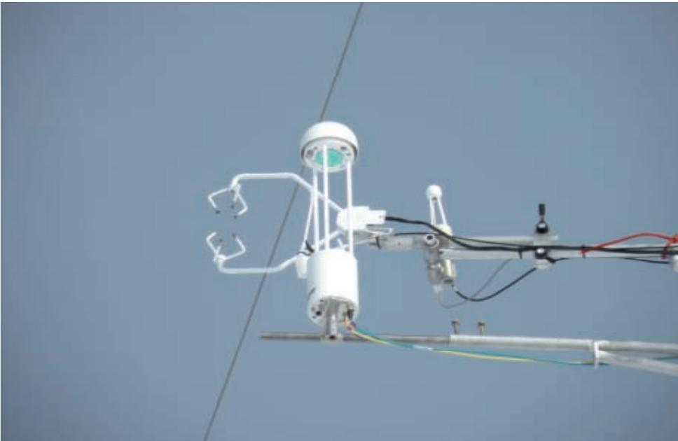
*Set up of the eddy covariance system and the open path gas analyzer at 20 m on the CCT*
