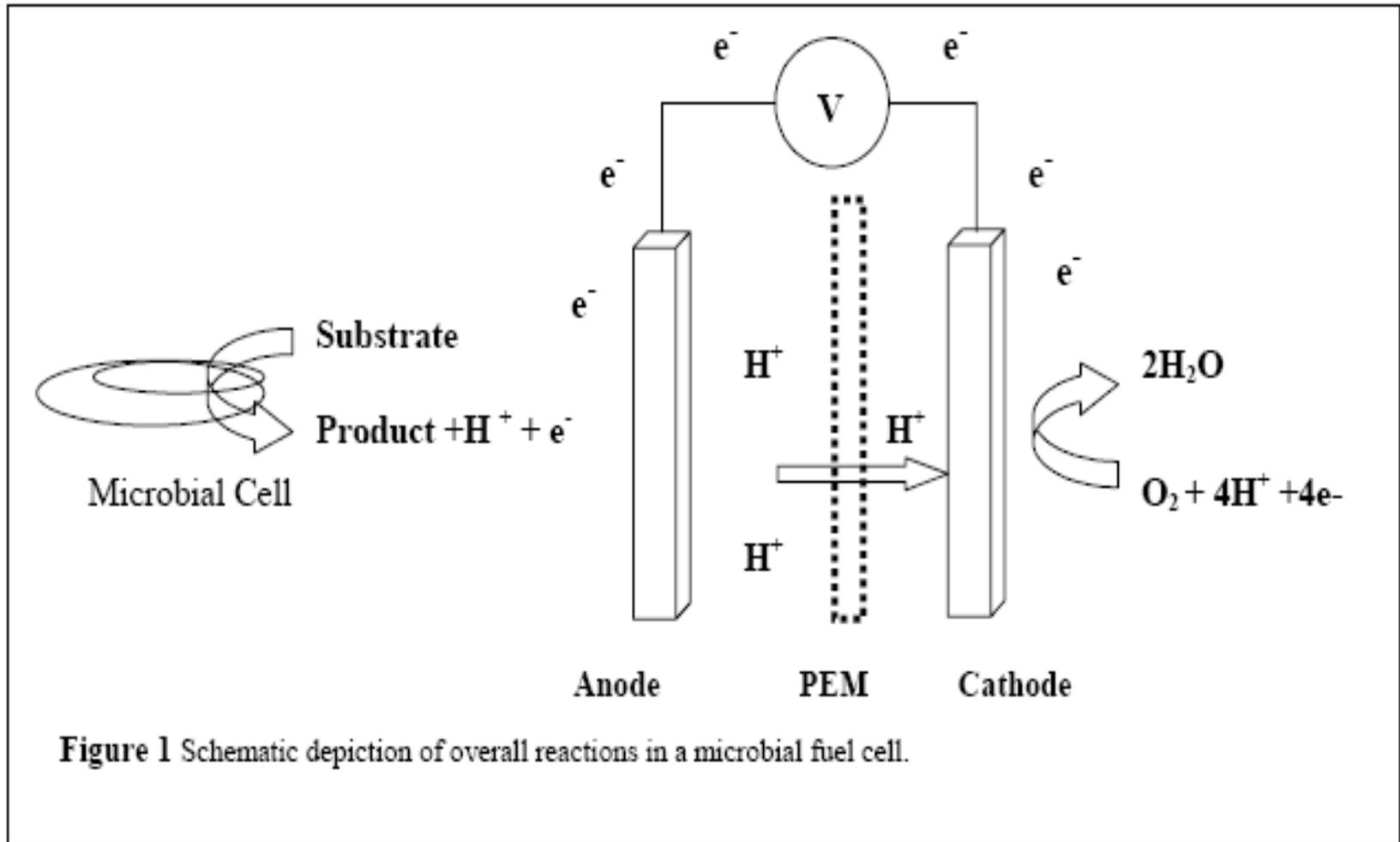
**Figure 1** Schematic depiction of overall reactions in a microbial fuel cell.
