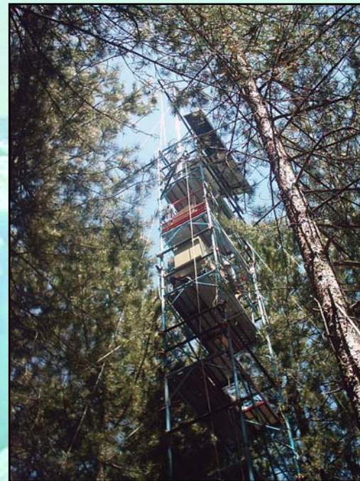
Infrastructure located in the Sila National Park for measuring carbon, water vapour and energy fluxes between forest ecosystems and the atmosphere. (Courtesy of Giuseppe Scarascia Mugnozza)
