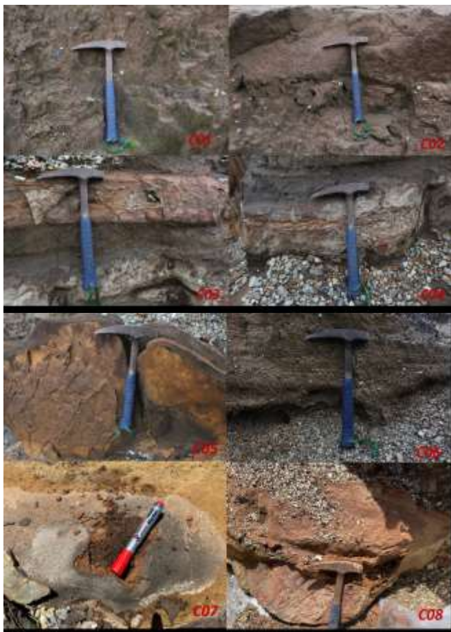
Ponente plant: tailing stratigraphy in the tailing dam
