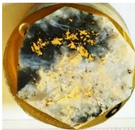
REE fluorocarbonates in quartz gangue – south from Gennamari
